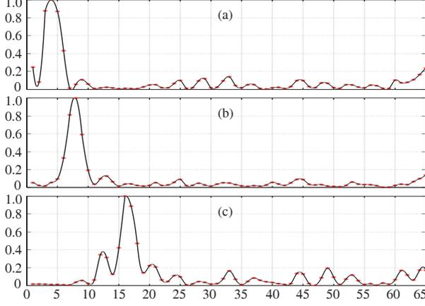
**Fig. 2.** The magnitude of the cross-correlation coefficients between: (a) the 4th and other frequency bins, (b) the 8th and other bins, (c) the 16th and other bins. The sampling rate is 8 kHz, the frame length is 16 ms (128 points), the FFT length is 128, and the overlap is 75%.
