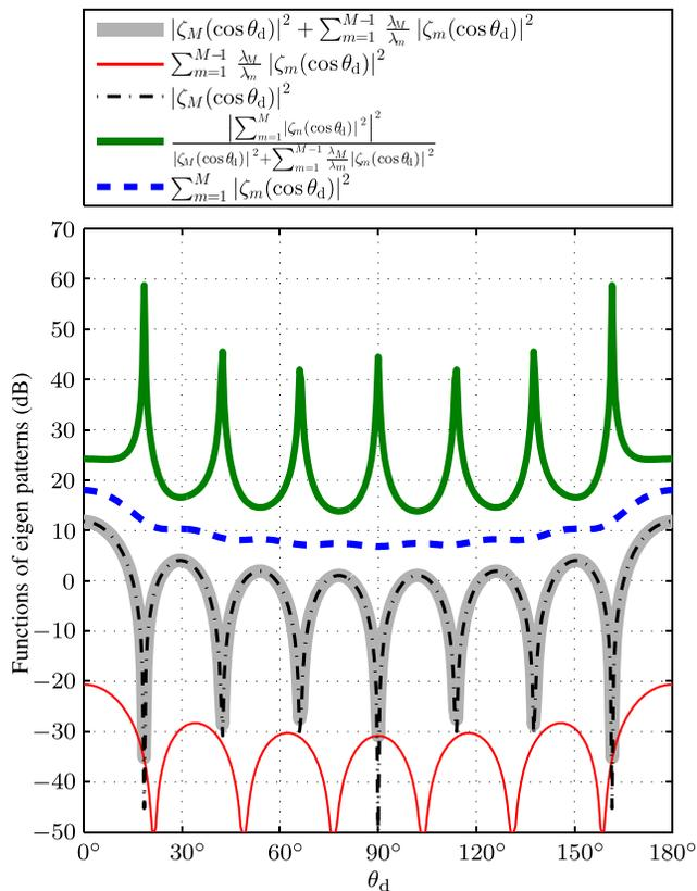
FIG. 9. (Color online) Illustration of the white noise gain of the conventional MVDR beamformer with a uniform linear array in diffuse noise:  $M = 8$ ,  $\delta = 2$  cm,  $f = 1$  kHz, and  $10 \log_{10}(\lambda_M) \approx -136$  dB.
