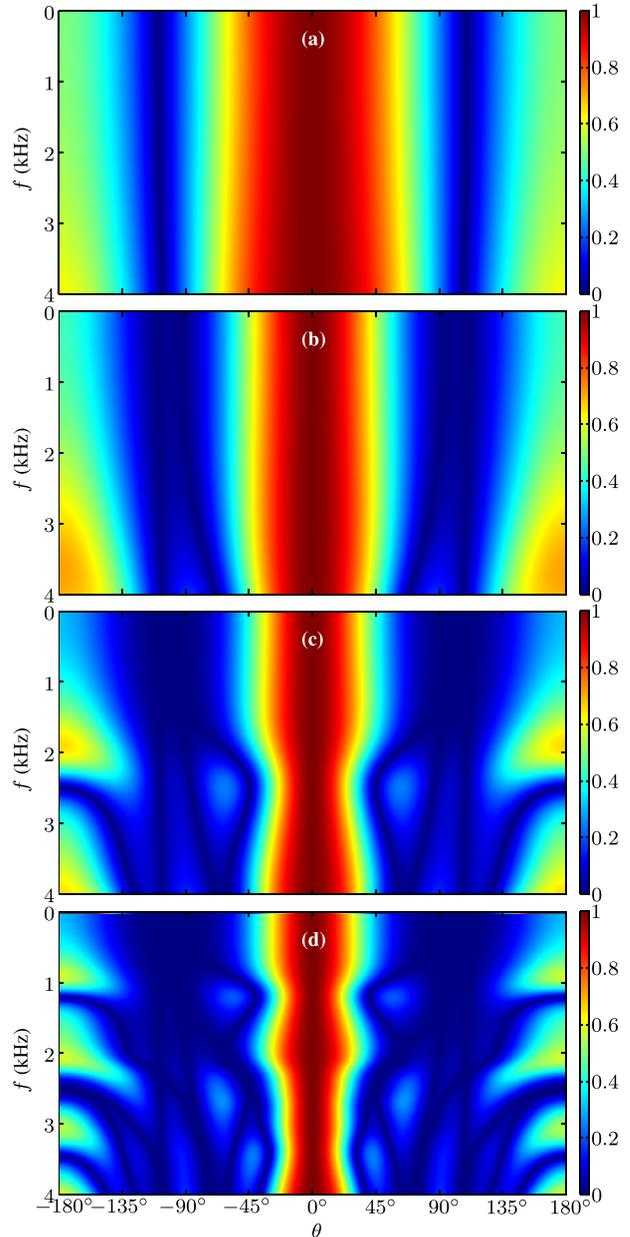
FIG. 7. (Color online) The noise spatial distribution of the multistage MVDR beamformer with a uniform linear array, 16 sensors,  $\delta = 2$  cm, and  $\theta_d = 0^\circ$ : (a) First stage, (b) second stage, (c) third stage, and (d) fourth stage.
