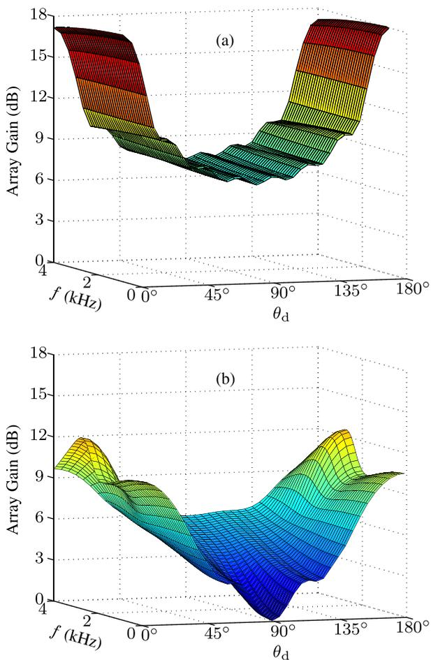
FIG. 4. (Color online) Array gain of the conventional and multistage MVDR beamformers as a function of frequency and source incidence angle with an eight-element uniform linear array ( $\delta = 2$  cm): (a) Conventional beamformer and (b) multistage beamformer.
